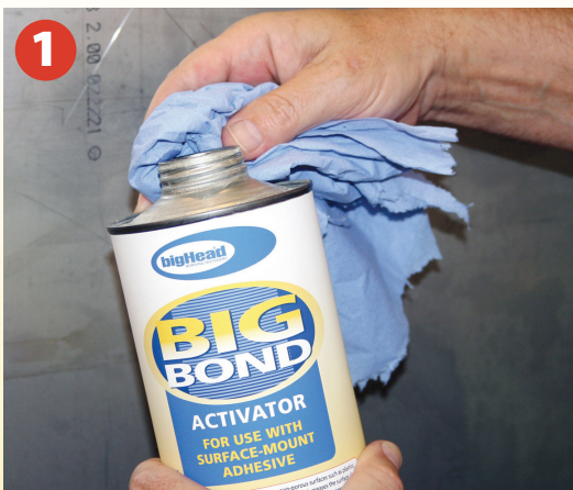
1 The surface (stainless steel is shown here) to take the BigHead must be clean and free of grease, oil, etc. We recommend using BigBond Activator/Cleaner for maximum performance.
