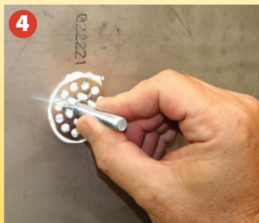
4 Press/rotate the BigHead firmly into the adhesive. Initial 'grab' is instant. Maximum strength takes up to 7 days of curing; increase in bond strength is progressive.
