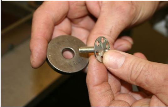
Loading fastener to test rig - Step 1
