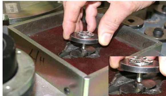
Loading fastener to test rig - Step 2
