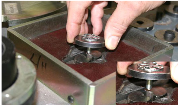
Loading fastener to test rig - Step 2
