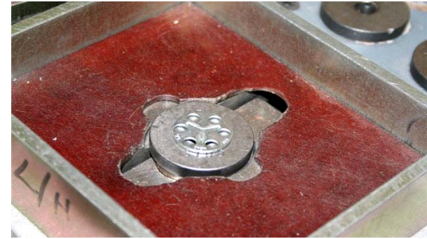
Loading fastener to test rig - Step 3
