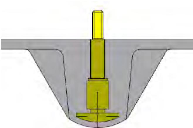
Alternatively, a bonding fastener such as a bigHead can be used, which is designed to be embedded in the composite material without the need for the material to be thickened. The thin flat head, shown in cross section below and which is perforated to allow the flow of composite material, helps transfer the load efficiently into the composite structure. The same threaded
